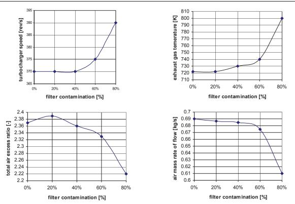
Fig. 1. Changes in selected marine engine parameters depending on the degree of contamination of the air filter
