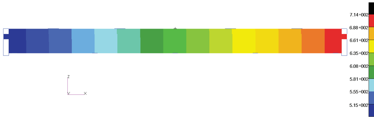
Fig. 6. Pontoons section immersion determined in numerical analysis
