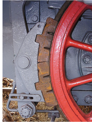
Fig. 2. The example of the railroad brake. Braking block (shoe) is seen next to wheel. (source: Internet)
