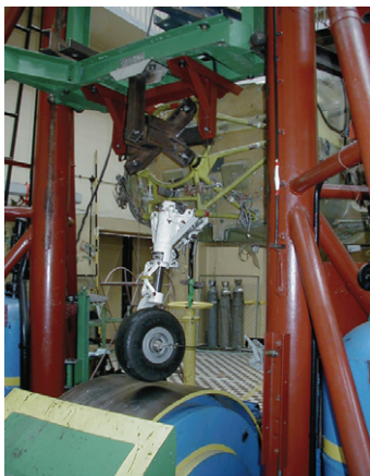
Fig. 7. Mlot 3T test rig for full scale brake testing with mounted airplane landing gear
