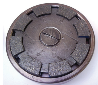
Fig. 6. Friction material mounted to test head of the IL68. (source: IoA)
