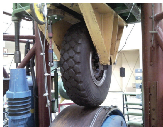
Fig. 8. Mlot 3T test rig with automotive brake and wheel mounted during tests
