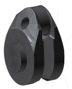
Fig. 1. Crankshaft FEM detailed model with one crank view
