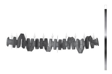
Fig. 5. Crankshaft deformation for elastic foundation
