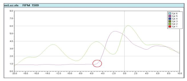
Fig. 6. Envelopes of vibration acceleration signals registered on the laboratory six cylinders diesel engine WOLA type 57H6Aa in "zoom" mode circle – angle of fuel velves open; engine speed = 1509 rpm, engine load = = 34 kW = 25% of nominal load
