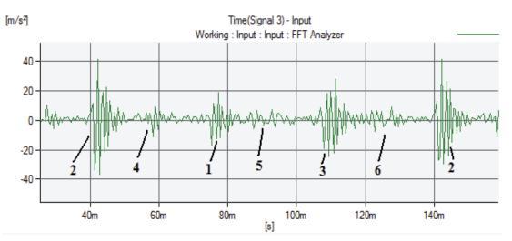
Fig. 2. Acceleration vibration signal measured on cylinder head number 2 in time domain. Engine firing order 1-5-3-6-2-4, plunger of the second section of fuel pump in normal operation
