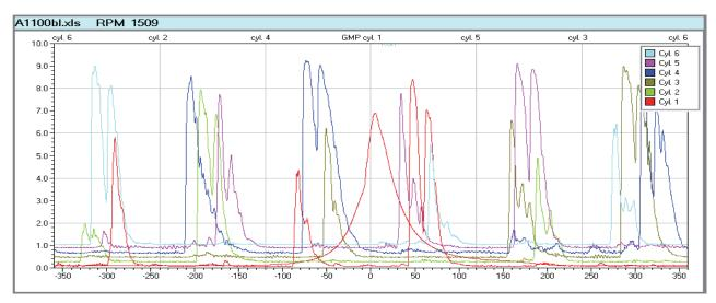
Fig. 7. Envelopes of vibration acceleration signals registered on one of the banks with six cylinders auxiliary diesel generator engine WOLA H12; engine speed = 1509 rpm, engine load = 100% of nominal load
