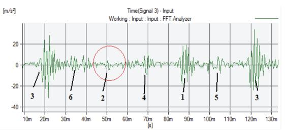
Fig. 1. Acceleration vibration signal measured on cylinder head number 2 in time domain. Engine firing order 1-5-3-6-2-4, plunger of the second section of fuel pump is blocked in upper position
