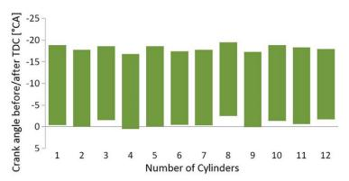
*Fig. 8. Values of fuel injectors angles of opening and closing for auxiliary diesel-generator engine WOLA H12; engine speed = 1500 rpm, engine load = 100% nominal load*
