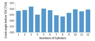
*Fig. 9. Values of intake valves angles closing for auxiliary diese-generator engine WOLA H12; engine speed = 1500 rpm, engine load = 100% of nominal load*
