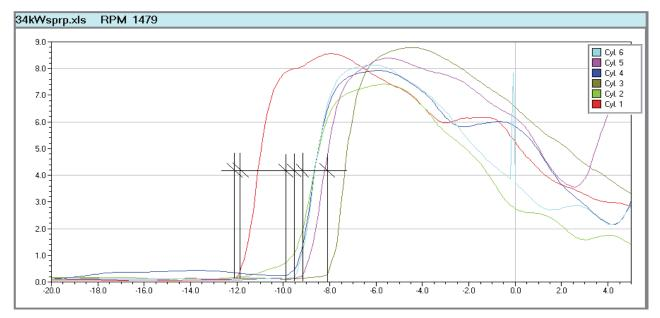
Fig. 4. Envelopes of vibration acceleration signals registered on the laboratory six cylinders diesel engine WOLA type 57H6Aa in "zoom" mode – angles of fuel velves opens; engine speed =1479 rpm, engine load = 34 kW = 25% of nominal load
