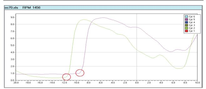
Fig. 5. Envelopes of vibration acceleration signals registered on the laboratory six cylinders diesel engine WOLA type 57H6Aa in "zoom" mode circles – angles of fuel velves opens; engine speed = 1456 rpm, engine load = = 34 kW = 25% of nominal load
