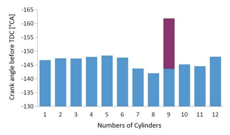
Fig. 10. Values of intake valves angles closing for auxiliary diese-generator engine WOLA H12; engine speed = 1500 rpm, engine load = 100% of nominal load
