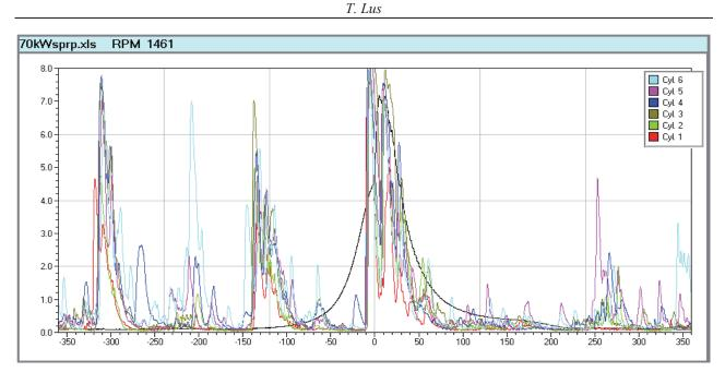
Fig. 3. Envelopes of vibration acceleration signals registered on the laboratory six cylinders diesel engine WOLA type 57H6Aa; engine speed =1461 rpm, engine load = 70 kW = 50% of nominal load
