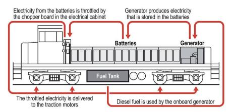
Fig. 6. A scheme of the hybrid technology applied in the Railpower GG20B Green Goat shunting locomotive [8]
