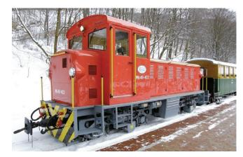
Fig. 11. Szilvásvárad Forest Railway Rába Mk 48 battery-hybrid locomotive [16]
