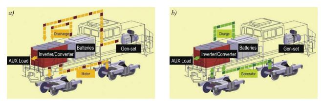
Fig. 2. Energy flows at powering (a) and breaking (b) mode for the HD300 hybrid locomotive [3]
