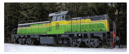
Fig. 3. The TEM9H Sinara Hybrid shunting locomotive [5]
