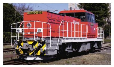
Fig. 1. Prototype of the Toshiba HD300 shunting locomotive [2]
