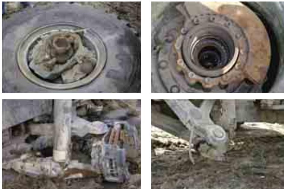
Fig. 10. Example of the impact of a reflected wave on the elements of the KTO Rosomak vehicle power transmission and suspension systems (photo: G. Motrycz).
