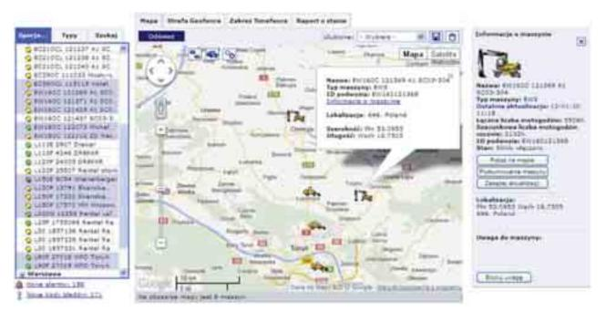
Fig. 2. Establishing the position of a selected vehicle with the use of a telematics diagnostic system
