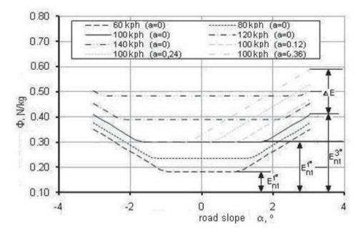
Fig. 5. The course of the unitary demand of the car energy-consumption at different constant speed and for instance for 100 kmph with different acceleration increasing  $\Delta E$
