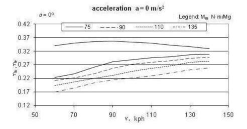
*Fig. 3.* The average efficiency of the passenger cars drive with the SI engines as a function of rational speed and dynamics of the drive in the phase with two drive phases
