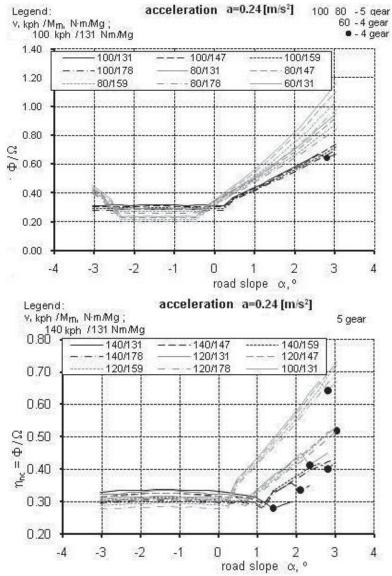
Fig. 6. The average efficiency vs. speed, dynamics and road profile with constant a=0.24 m/s<sup>2</sup> speed profile
