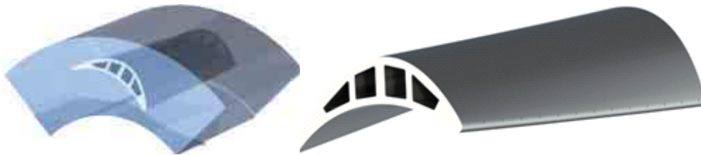
Fig. 3. On the left - placement of airfoil in the hot gas channel, right - airfoil with cooling geometry
