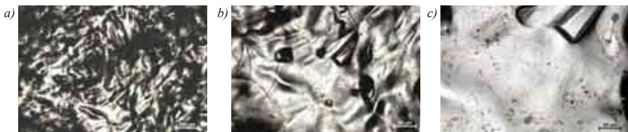
Fig. 2. MM images of 1 (CuZnNi) sample surface: a) the scale of 100 \mu m, b) the scale of 50 \mu m, c) the scale of 20 \mu m
