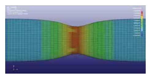
Fig. 12. Map of effective strain in the neck area from FEM analysis
