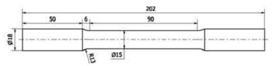
Fig. 1. Scheme and overall dimensions of the tensile specimen
