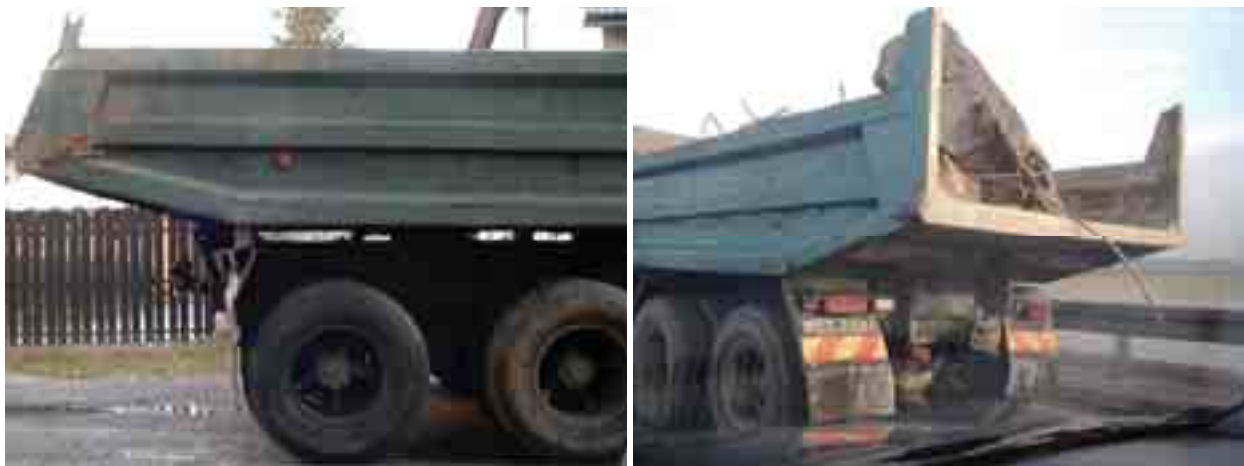
Fig. 14. The examples of protruding of bodies of the self-unloading trucks
