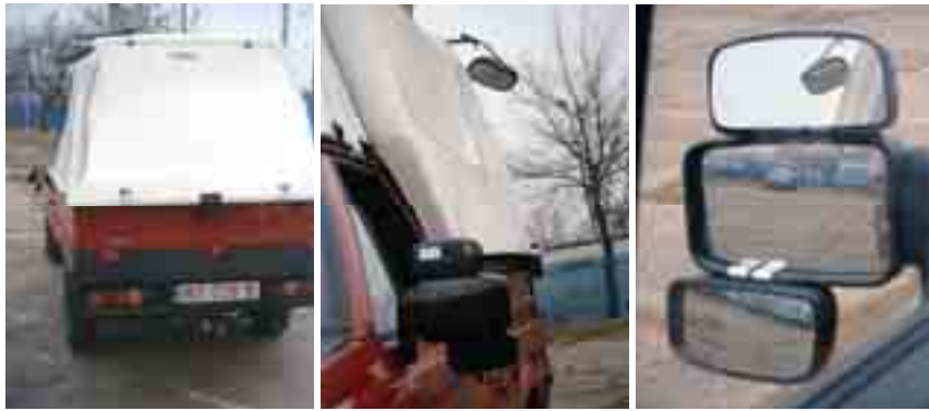
Fig. 1. The placement of the mirrors in the tested vehicle, view from outside of the left side of the vehicle (from the back and from the front) and the view from the place of the driver to the left through the window of the left door
