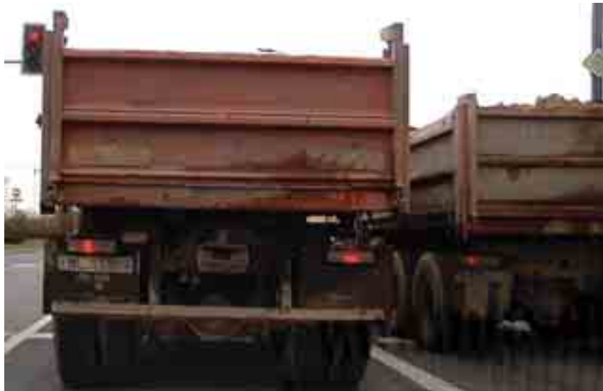
Fig. 15. The examples of the self-unloading vehicles of the same make and type with / without the rear under run protection
