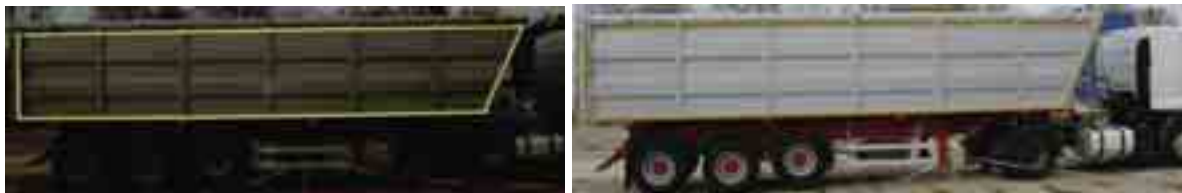
Fig. 9. The view of the semi-trailer, the placement of the sidelights and contour marking - the view in the artificial and daily light
