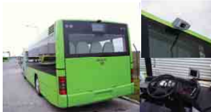
Fig. 11. The view of the bus, the placement of the camera and the screen of the projector in the cab
