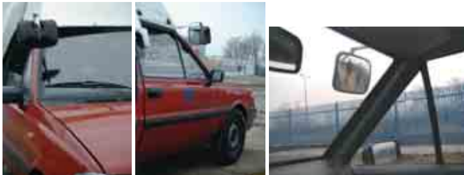
Fig. 2. The placement of the mirrors in the tested vehicle, the view from outside of the right side of the vehicle and the view from the driver's place to the right on the right pile A
