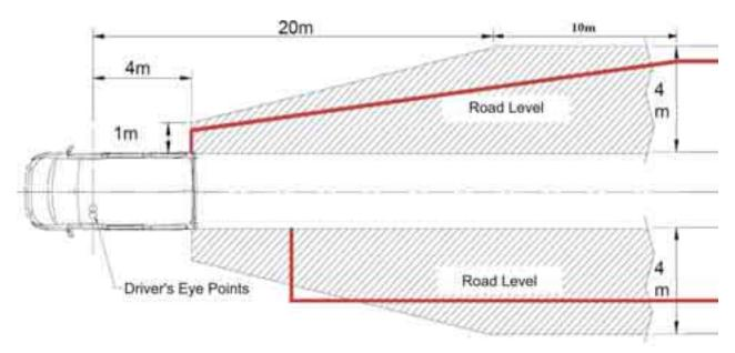
Fig. 3. Placement and vastness of the visibility field for the main rear view mirrors of class III – by thickened line denotes requirements hitherto in force -  $dmc \ge 2000 \text{ kg}$  [3]
