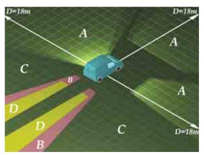
Fig. 2. The areas around the vehicle category N1 which are visible
