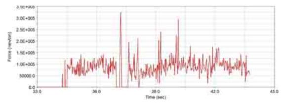
Fig. 13. The change of the contact force in the tailboard joint – velocity 115 km
