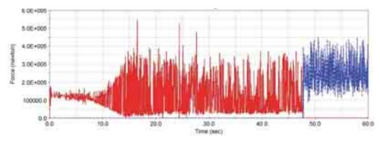
Fig. 10. The resultant change of force value of wheel – rail contact during the transit at 60 km/h velocity
