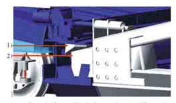
Fig. 5. Lock connecting tailboards of rotatable platform and a part of frame: 1) wedge, 2) lock-hook
