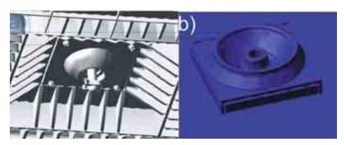
Fig. 4. Model of swivel pin used as central junction of floor rotation a) loading floor – down view, b) support – top view
