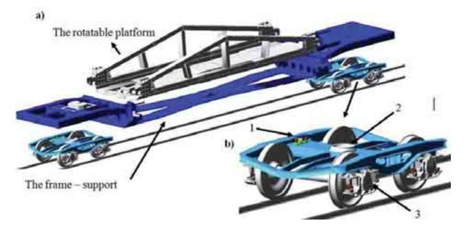
Fig. 2. a) Chart of 3D numerical model with main subsystems, b) Y25 type bogie 1- side slides, 2- swivel pin, 3-spring element of bogie suspension
