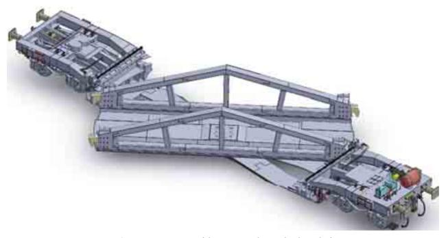
Fig. 1. Prototype version of the wagon with open loading platform
