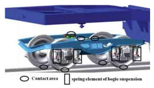
Fig. 3. Charts illustrating constraints and conditions of cooperation (contact) in connections of subsystems of bogies, frame-support and central junction
