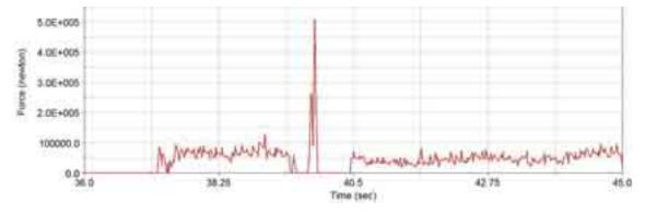
Fig. 12. The change of the contact force in the tailboard joint – velocity 90 km
