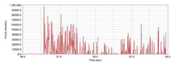
Fig. 11. The change of the contact force in the tailboard joint – velocity 60 km
