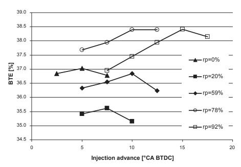
Fig. 2. Brake thermal efficiency in the function of injection advance at different premixed ratios [29]
