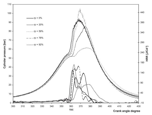
Fig. 4. Cylinder pressure curves and heat release rates in the function of crank angle at 100% load and injection advance of 7.5 CA° BTDC [29]
