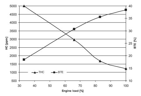
Fig. 3. HC emission and brake thermal efficiency vs. engine load at nearly constant pilot dose (0.46-0.60 [kg/h]) [29]
