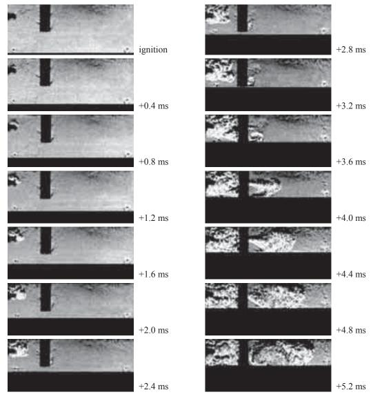
Fig. 17. Combustion process in a model combustion chamber during the tests using RCM:  $V_{kw} = 28\%$ , d = 3 mm, ignition at the prechamber wall,  $\varphi_{wz} = 45^{\circ}CA$  BTDC
