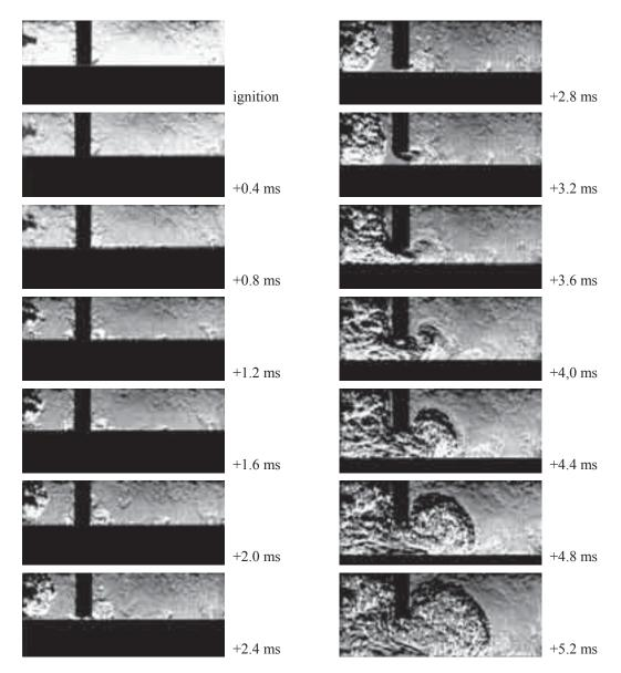
main combustion chamber, followed through the clearance and the combustion mechanism in this system was different from demanded, and the system performance was similar to the standard design.
