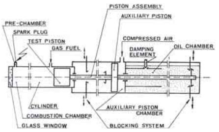
Fig. 1. Pneumatically driven RCM schema
