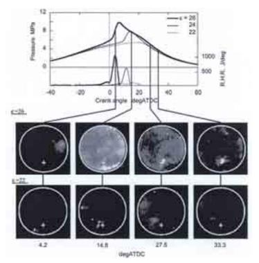
Fig. 9. Effect of compression ratio on HCCI combustion [1]
