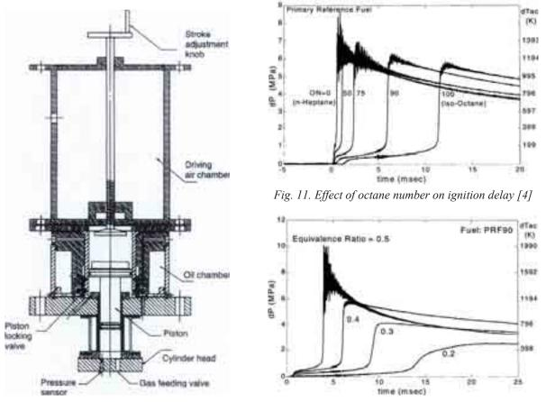
HCCI engines. Fig. 11 shows the combustion histories of the fuels with different octane number: 0 (n-heptane), 50, 75, 90 and 100 (iso-octane).
