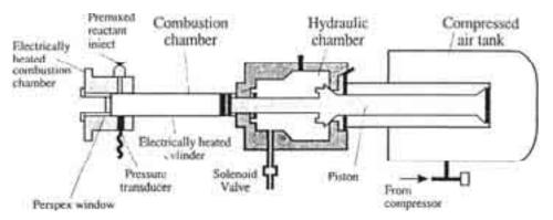
Fig. 4. RCM schematic with pneumatic drive, used by Griffiths and Kordylewski [3]
