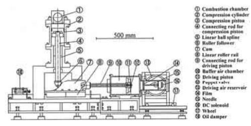
*Fig. 5. Murase RCM used in research of pulsed jet combustion [6]*
