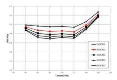
Fig. 9. The simulation computations concerning the influence of the change in the solid cell packing density at a constant solid volume of 1.4 dm<sup>3</sup> on the change of the content of NO in  $NO_x$
