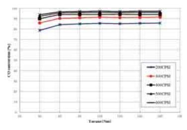
Fig. 7. The simulation computations concerning the influence of the change in the solid cell packing density at a constant solid volume of 1.4 dm³ on the change of the CO conversion
