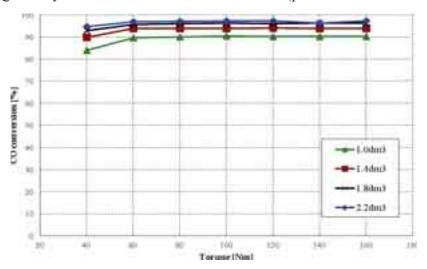
Fig. 3. The simulation computations concerning the influence of the change in the reactor solid volume at a constant cell packing density of 400 on the change of the CO conversion
