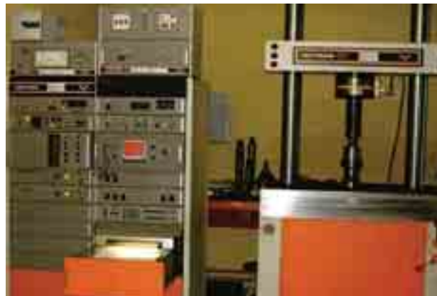
Fig. 7. Endurance machine static-dynamic of type Instron 1273
