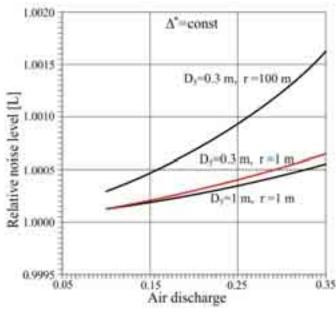
Fig. 9. Ratio of the levels of noise of the engines: two-flow engine equipped with air stream flow mixing device and the "bypass" type of engine depending upon the amount of air flowing through the external ducts of both engines and the radius r as well as upon the diameter of the discharge nozzle  $D_5$ .
