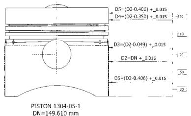
Fig. 3. Design of the 1304-05-1 novel piston
