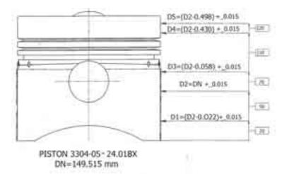
Fig. 1. Design of the 3304-05-24.01BX standard piston
