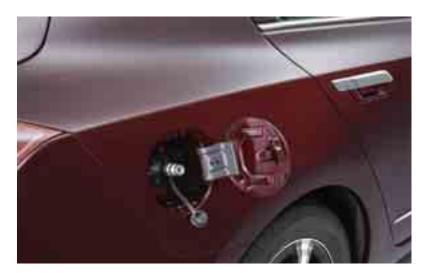
Fig. 1. Honda's FCX Clarity hydrogen tank inlet
