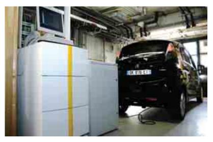
Fig. 2. An Electric Vehicle (right), charged from a stationary "early market" commercial SOFC power unit (middle). This SOFC also "transfers" the waste heat to the domestic water tank (left)
