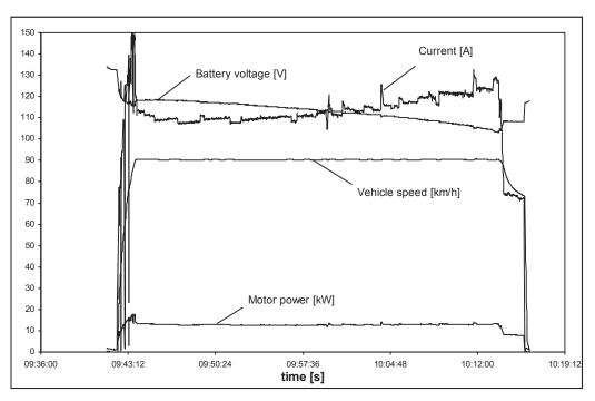
Fig. 6. The test at a speed of 90 km/h
