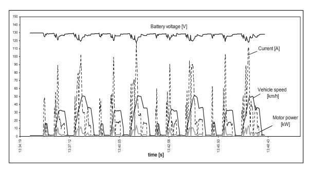
Fig. 11. The parameters of the selected NEDC test
