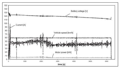
Fig. 12. The parameters of the selected test at 60 km/h, in accordance with the record AR205\_0\_2011-01-26\_14-07-22
