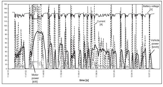
Fig. 8. FTP test parameters after charging the batteries. The record file AR205\_0\_2011-01-17\_11-44-49
