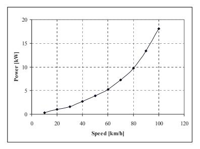
Fig. 4. The average electric power versus vehicle
