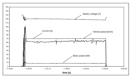
Fig. 5. The test at a speed of 70 km/h
