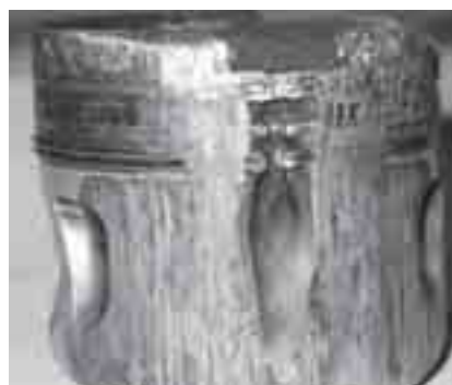
Fig. 6. Removal of material by melting on the piston crown
