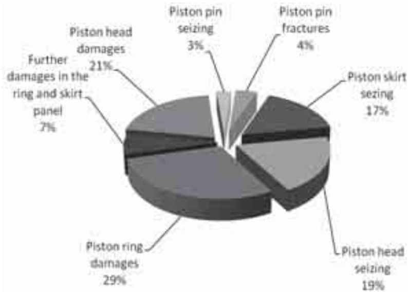
Fig. 2. Structure of piston damages
