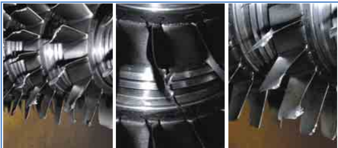
Fig. 1. Characteristic damage of GTD-350 engines
