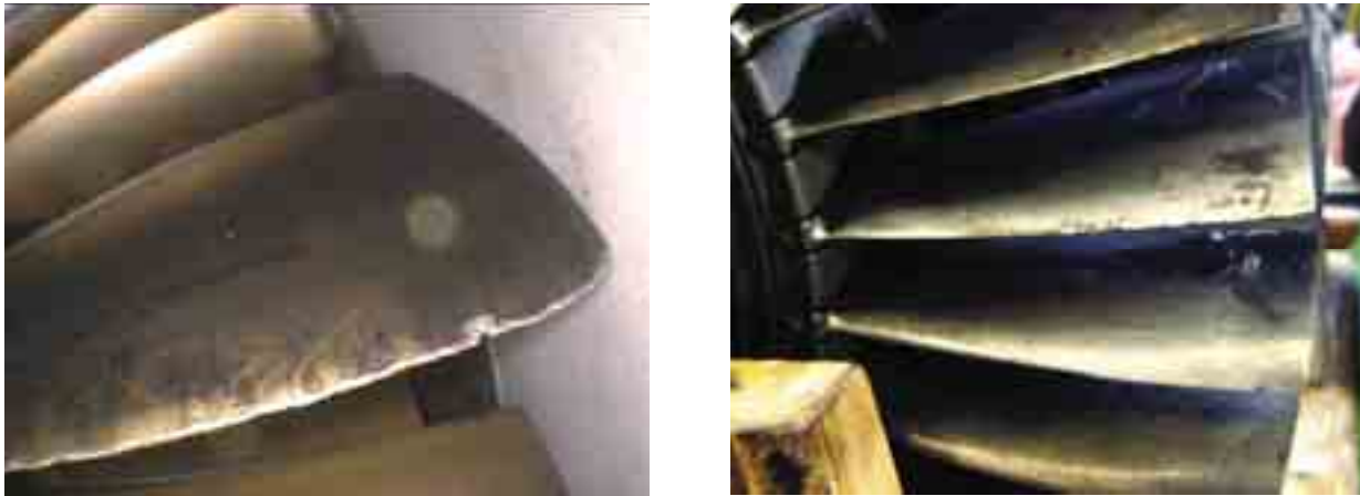
Fig. 4. Damaged areas and erosion on leading edges of the compressor first stage rotor blades
