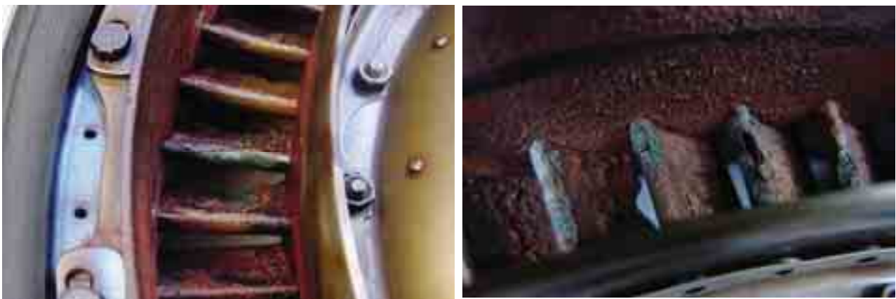
Fig. 5. Damaged areas (overheat, damage of the calorisation layer, material losses, deposit of burnt sand) on the compressor first stage guide vanes
