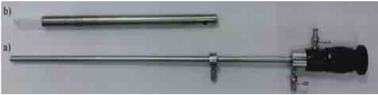
Fig. 2. a) Endoscope of the unit AVL Engine VideoScope 513D, b) Quartz shield/housing of the endoscope end
