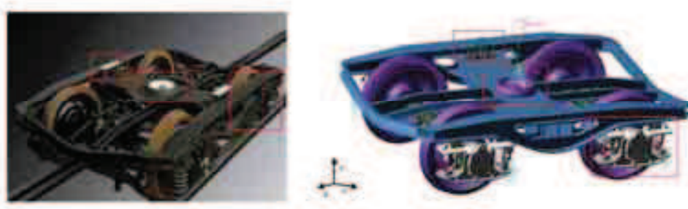
Fig. 4. Actual trolley Y25 [9] and its corresponding numerical model [1]
