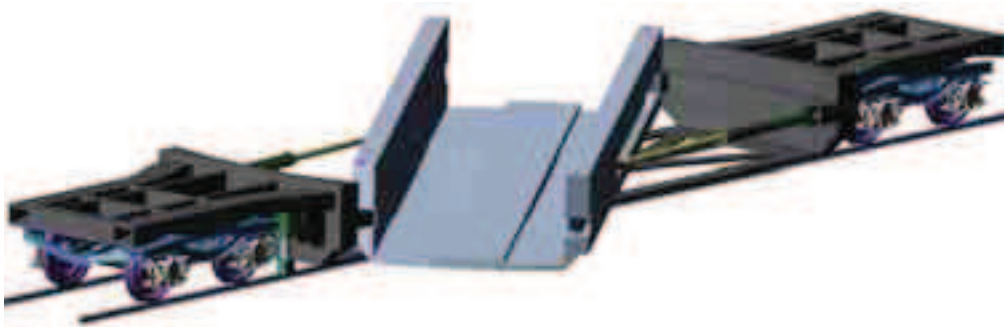
Fig. 3. Numerical model of railway wagon adopted for analyses [1]
