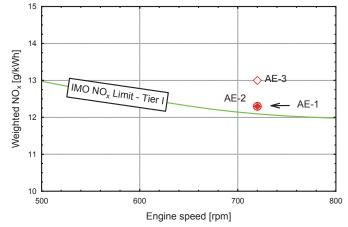
Fig. 7. NOx emission factors for ship diesel engine generators in Tier 1 limit
