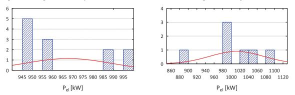
*Fig. 8. Electric load histogram while berthing in the port; Świnoujście (left diagram) and Ystad (right diagram)* Operating costs connected with the ship electric energy generation can be reduced at this
