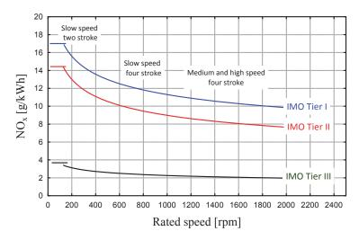
Fig. 1. Nitrogen oxides emission limits for marine engines
