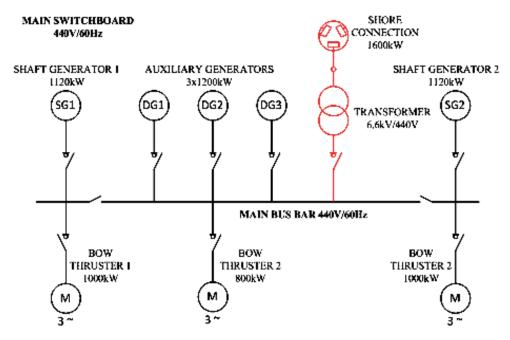
Fig. 5. The configuration of the electric supply system with the planned shore connection (in red)
