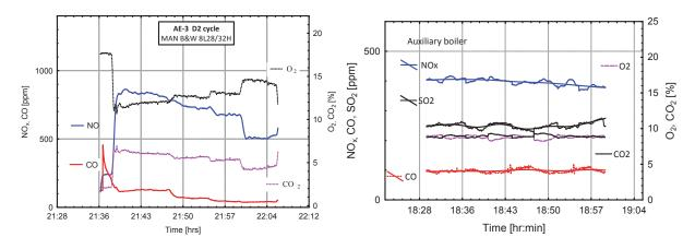
Fig. 6. The exemplary, registered exhaust gas composition for engine AE 3 and heating boiler
