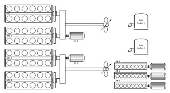
Fig. 4. The scheme of configuration for the main and auxiliary propulsion of m/f Skania
