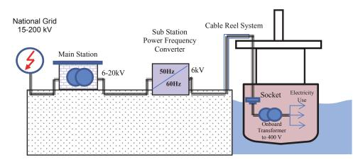
Fig. 2. The scheme of vessel electric supply system configuration in the port according to EU regulations
