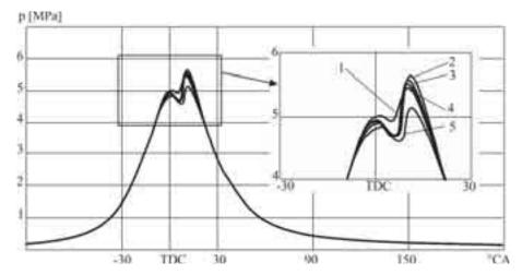
*Fig. 1. Average changes of pressure in the combustion chamber at double-fuel engine fuelled with diesel oil (DO) at a varied constant angle of pilot dose injection of 20°CA, at Ne=2kW, N=3000 rpm, and various shares of methane in the dose powering the engine: 1 – 100% DO, 2 – 50% DO+CNG, 3 – 33% DO+CNG, 4 – 22% DO+CNG, 5 – 12% DO + CNG*
