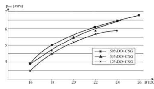
*Fig. 3. The effects of advance angle of the pilot dose injection on the maximum pressure of combustion, at various proportions of diesel oil and CNG*
