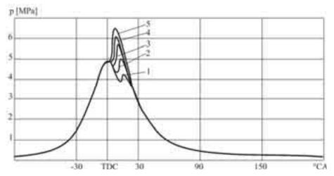
Fig. 2. Average changes of pressure in the combustion chamber at dual fuel engine supply with diesel oil at varied pilot dose injection angle, at Ne=2k, N=3000 rpm, a dose of diesel oil of 22%: 1 – 16°CA, 2 – 18°CA, 3 – 20°CA, 4 – 22°CA, 5 – 24°CA
