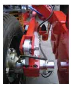
Fig. 2. Measurement wheel of dynamometer trailer
