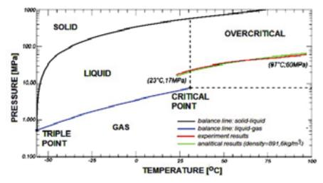
Fig. 6. Comparison of analytical and experimental tests of CO<sub>2</sub> heating
