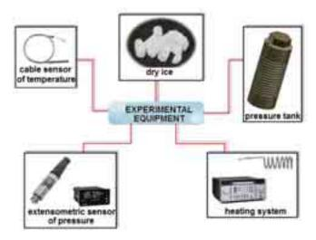
Fig. 5. Research equipment for CO2 thermodynamic behaviour testing
