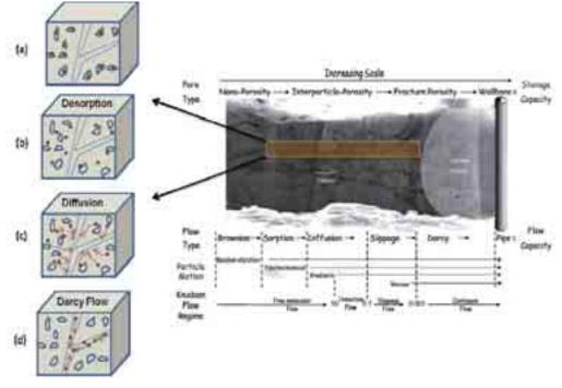
Fig. 2. Flow types and behaviour in shale reservoirs [10]
