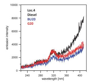
Fig. 8. UV emission spectra detected at 0.8 CAD ASOC in central location of the combustion chamber (SOI=11 CAD BTDC, EGR%=0)
