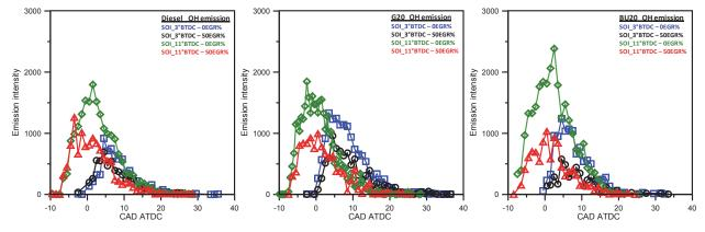
Fig. 11. OH evolution evaluated from spectroscopic measurements for the conditions with SOI = 11 CAD BTDC and 3 CAD BTDC
