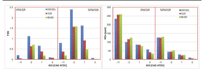
Fig. 3. Engine exhaust emissions of soot (filter smoke number - FSN) and NOx vs. the start of injection (SOI) for all the operative conditions
