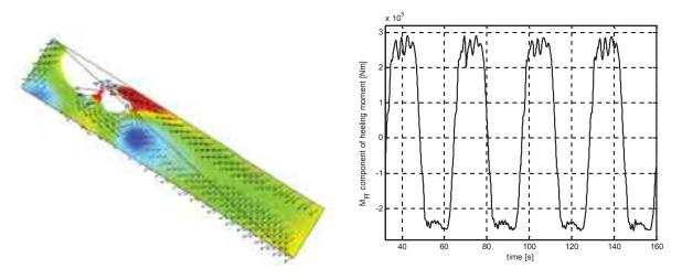
Fig. 9. Results of CFD computation – velocity field and vectors (left) and a history of heeling moment due to liquid sloshing in the considered tank (right)
