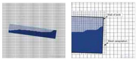
Fig. 6. Mesh applied for CDF calculations
