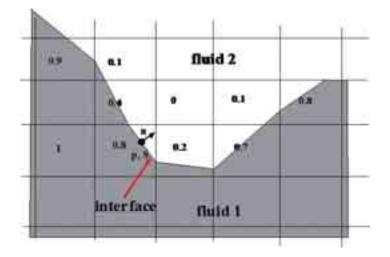
Fig. 8. VOF (Volume Of Fluid) variable is the volume fraction of fluid 1 in a cell, VOF=1 - the cell contains only fluid 1, VOF=0 - the cell contains only fluid 2, 0<VOF<1 the cell contains fluid 1 and fluid 2 [1]
