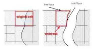
Fig. 7. Sub-grid resolution of curvilinear wall [1]
