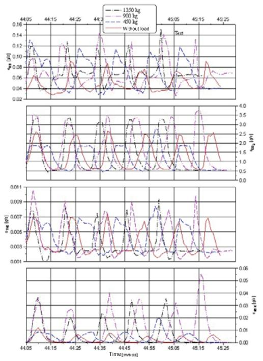
Fig. 2. The course of pollutants emission intensity from a forklift truck during lifting loads of different weights
