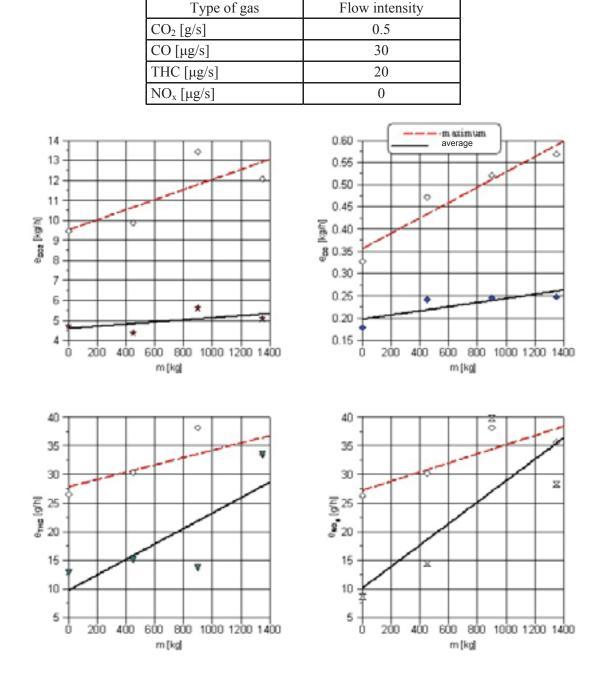
Tab. 2. The intensity of the emission of exhaust components during the forklift truck engine idling
