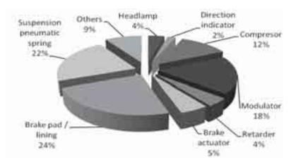
Fig. 4. Structure of faults of particular parts for busesM3/III
