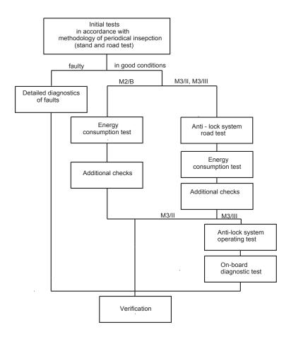
Fig. 1. Algorithm of vehicle examinations
