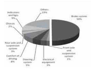
Fig. 2 Structure of vehicle faults
