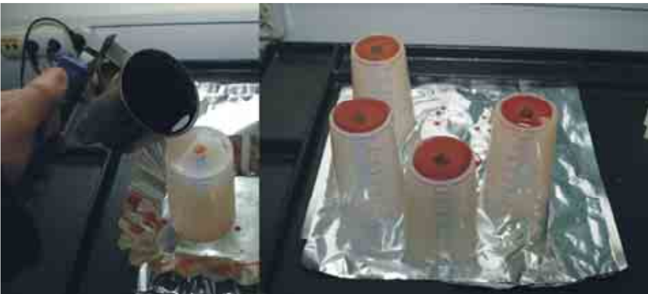
Fig. 5. Silicone mould pouring cylinder core wax model
