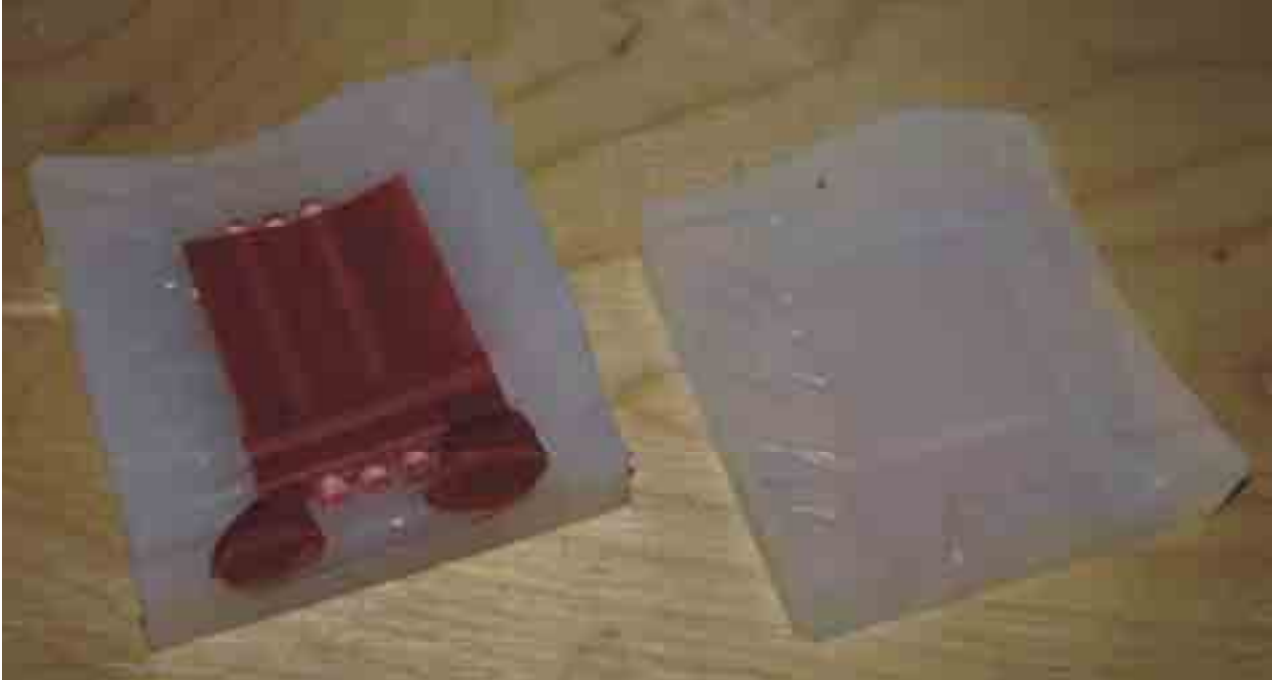
Fig. 4. Wax model of core blade and silicone mould
