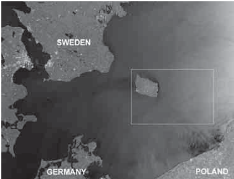
Fig. 2. Exemplary SAR-image for Southern Baltic Sea. Image obtained from CleanSeaNet [7] and processed by the author (contrast adjusted to the area near the Polish coast). Several other oceanological phenomena like upwelling and oscillations of atmospheric pressure close to seashore in the lower part of the picture are visible
