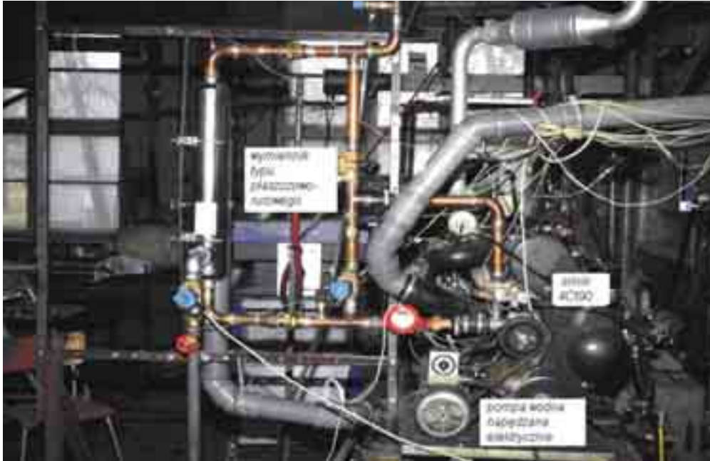
Fig. 2. Engine 4CT90 on the dynamometer with cooling system pressure
