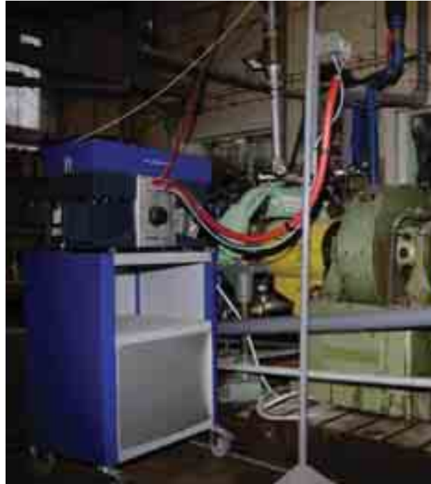
Fig. 1. Measurement of smoke opacity by means the opacimeter AVL-486
