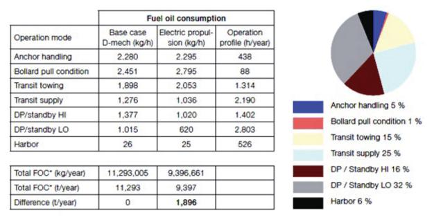
Fig. 5. Comparison of fuel oil consumption for two types of main propulsion: electric propulsion and direct mechanical propulsion for a 200+ ton bollard pull AHTS [3]
