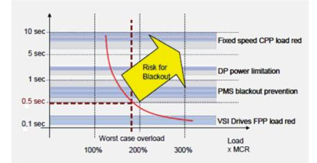
Fig. 3. Risk for blackout of different power management systems and level of overloading [9]
