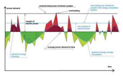
Fig. 4. The power demand with energy accumulation method
