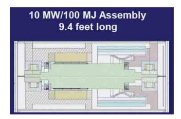
Fig. 9 Reacon POWER proposition of fluwheel for naval ship of 10 MW (27.8 kWh) [8]
