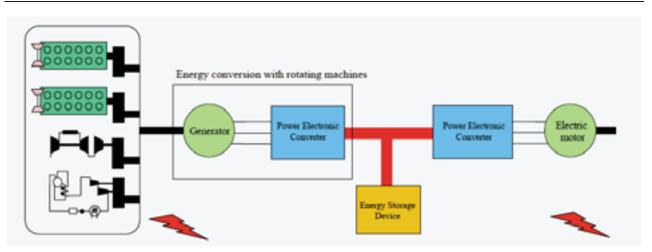
Fig. 1. Structure of combined ship's power plant [1]
