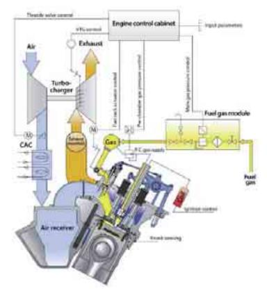
*Fig. 3. Supplying fuel system of Bergen gas engine [1]*
