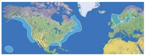
Fig. 1. IMO and EPA emission controlled areas [1]
