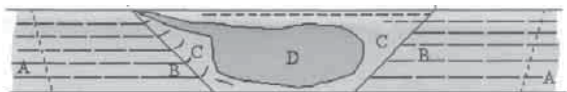
Fig. 1. Schematic diagram of the FSW joint structure welded on one side [P1]
