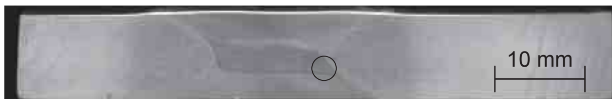
Fig. 2. Macrostructure of FSW welded joint (double-sided welding) - marked by circle welds fragment selected for microscopic examination
