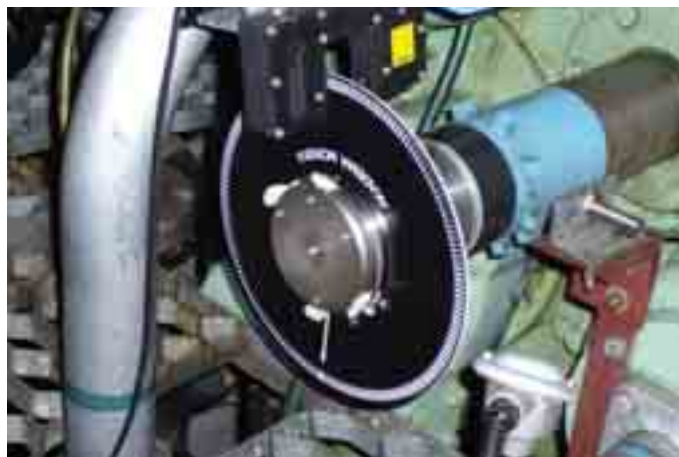
Fig. 4. Measurement disc and laser sensor mounted at crankshaft free end
