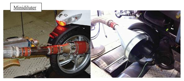
Fig. 1. Passage of exhaust gas from tailpipe to CVS: closed (left), open (right)
