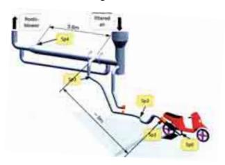
Fig. 3. Sampling positions (Sp) used in the tests
