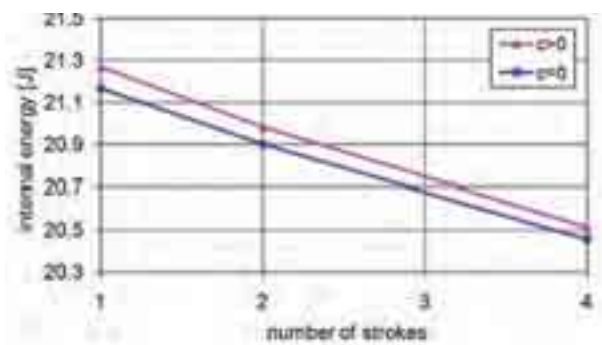
Fig. 8. Strain rate influence on the rivet internal energy
