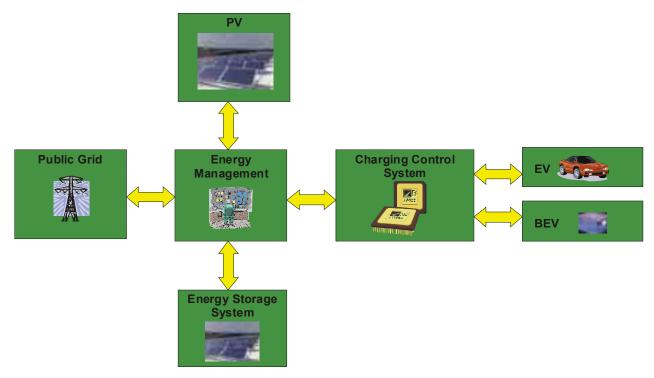
Fig. 1. Scheme of the charging station operation
