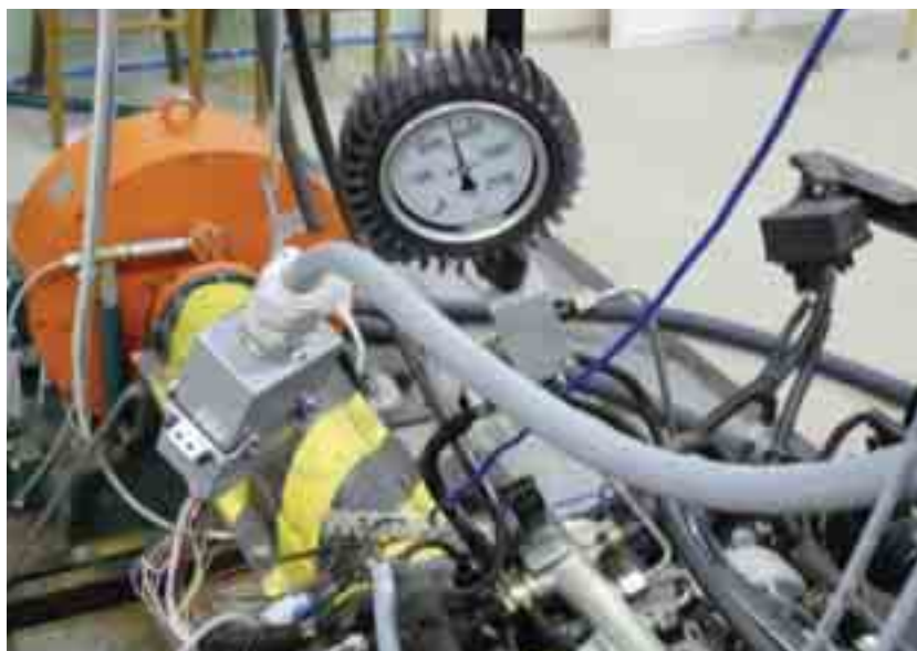
Fig. 2. Pressure gauge for testing Common Rail high-pressure on FIAT 1.3JTD engine
