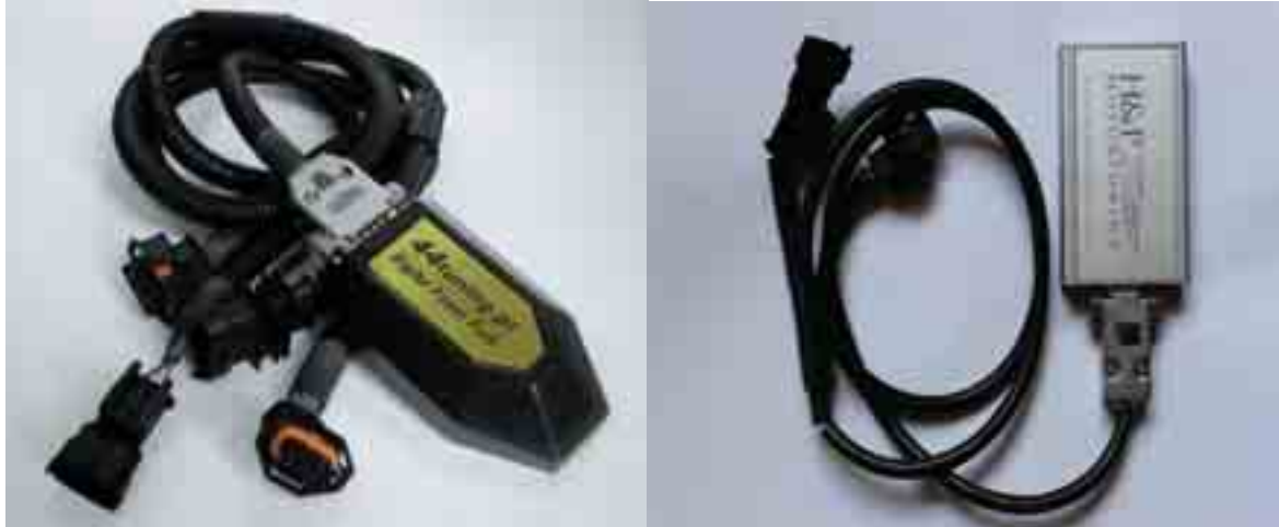
Fig. 5. Box of the Digital Power Pack type (DPP - left) and classic box (right) [7]
