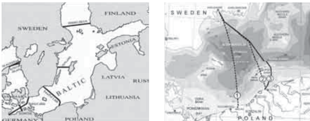
Fig. 3. High voltage electric power cables in the Baltic Sea (left), changes of SwePol Link routs due to protests of local communities and nature conservation issues (route No.1- original proposal: one cable and two electrodes, route No. 2 – second proposal: main and return cable replacing electrodes, route No. 3 - adopted solution: cable route avoiding stony reefs of the Slupsk Bank (right)
