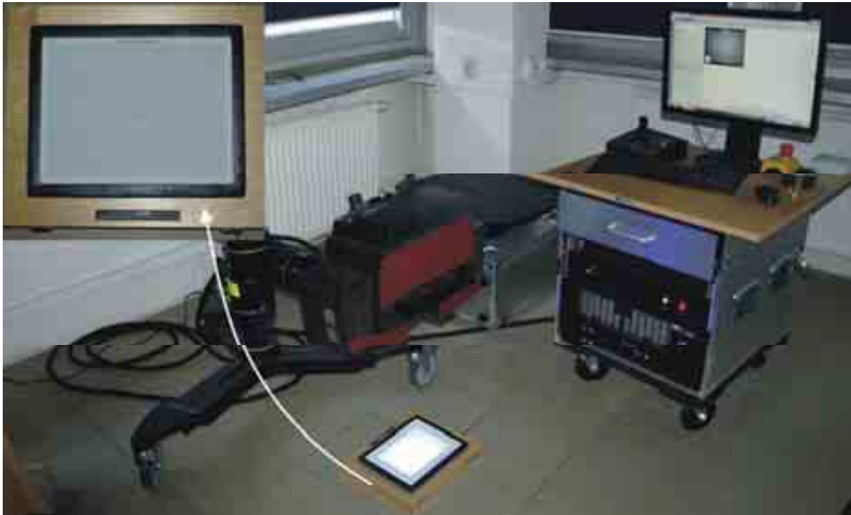
Fig. 2. Calibrations of GOM ATOS II Blue Light scanner
