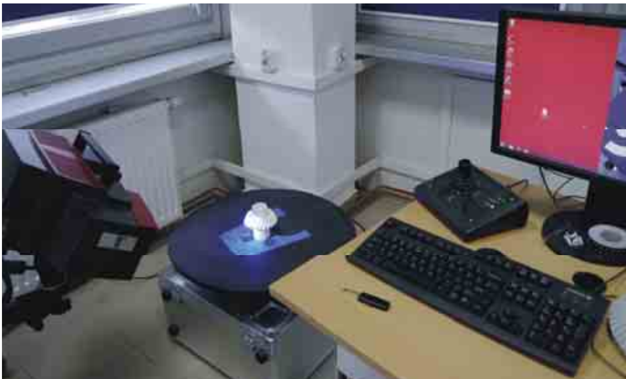
Fig. 1. The measuring system GOM ATOS II Blue Light
