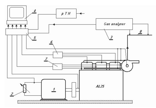
*Fig.1.* The laboratory stand scheme. 1 – generator, 2 – water resistance, 3 – gas analyser, 4 – computer, 5 – *A/C* converter, 6 – combustion pressure indicator, 7 – injection pressure indicator, 8 – exhaust duct
