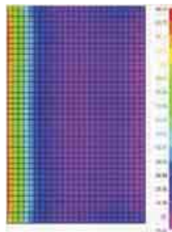
Fig. 15. Distribution of maximum principal stresses in adhesive layer of double lap bond subjected to shearing
